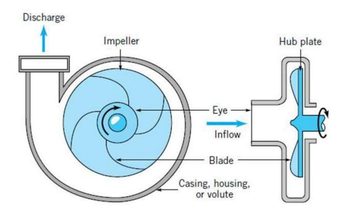
Centrifugal pumps are widely used in STPs to move water and sludge. They convert rotational energy into fluid flow.
